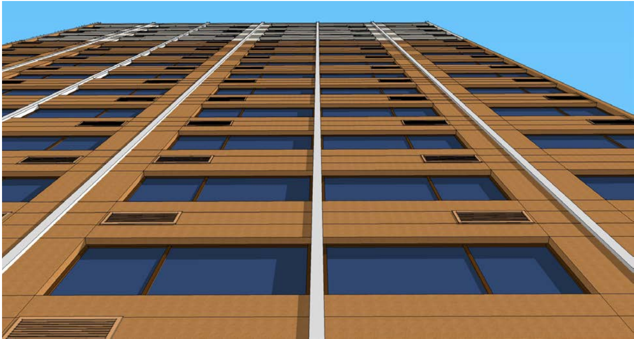
Figure 18 – Scheme C1 Façade – Terracotta Panels
