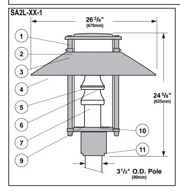
Fixture Cover - Aluminum cover with white painted interior for maximum fixture efficiency, has industrial felt gasketing for air circulation. Cover removes for lamp access. 2. Cover Support - Machined support connected to fixture cover with architectural Allen head nut detail.
