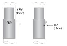
**GFCI Receptacle (REC)** - GFCI duplex receptacle with cast base bolted to pole and gasketed, provided with weather-proof, self-closing cover; located 36" (915mm) from base of pole, inline with handhole. Receptacle is intended only for portable tools or other portable equipment to be connected to outlet only when attended by operating personnel.
