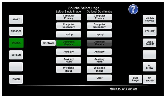
Source Select page for rooms with two displays. If a room has two "main" displays, the display to the audience's left (stage right) is "Display 1" and the display to the audience's right (stage left) is "Display 2"
