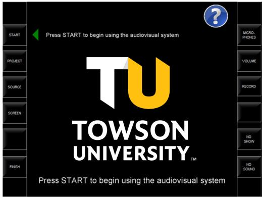
3. Start (If the START button is pressed and the user does not press PROJECT to continue with startup it must return to the splash screen in 30 seconds.)
