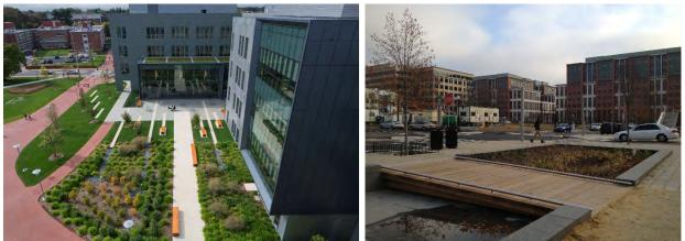
Examples of how bioretention facilities can be incorporated into plaza designs.
